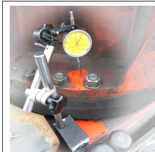
Dial gauge in measurement position
